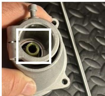
8. You now can slide this back over the drive tube seating the splines and replacing the 2 bolts and washers from the other housing. Make sure you use the same alignment hole and snug up the bolts. Do not overtighten these bolts. Aluminum is not as hard as stainless steel and will strip if forced too hard.
