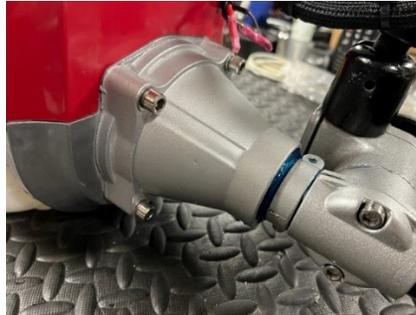
3. Unbolt the 4 engine bolts loosening as you go, and then fully removing them.
