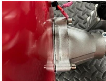
4. You will slide the motor away from the clutch housing and rest it on the clutch so it doesn't wobble around.
