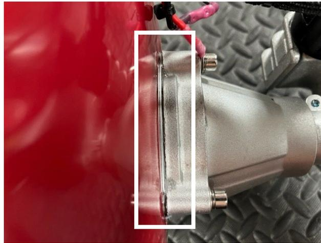
12. Before you snug up the engine leave about 3-5mm space and add a bead of RTV sealant around the surface of the where the clutch housing meets the engine block. Think of this as a gasket to keep any dripping water from entering.
